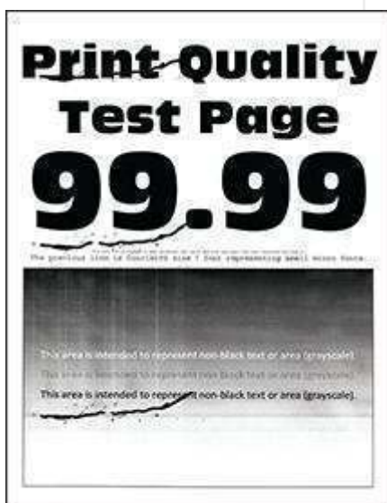
Repeating defects on page 717
