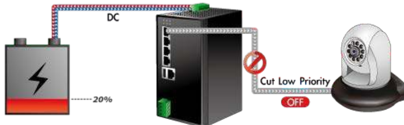
Figure 4-5-3 Low Voltage Cut-Off Protection
