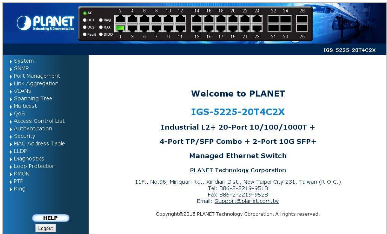
Figure 3-4: Web Main Screen of Industrial Managed Switch
