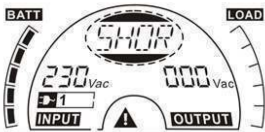
■ Figure 6.5 The Fault mode
