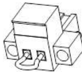
Figure 23: Emergency power off connector
